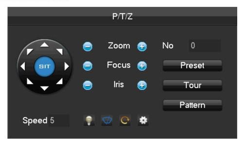
Direction, steps, zoom, focusing, iris, preset points, cruising between points, patrols, sweeping the boundary, calling an auxiliary switch, light switch, horizontal rotation of PTZ can be controlled.
