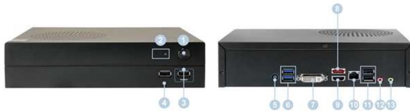
Figure 1-1. Front & Rear View of NR-1100 Series
